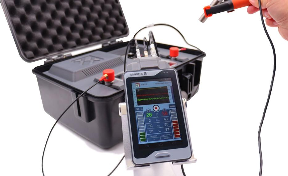
**Figure 3:** Multi-channel test device with two ultrasonic sensors and one rotation speed sensor on the bearing demonstrator. Photograph: SONOTEC.
