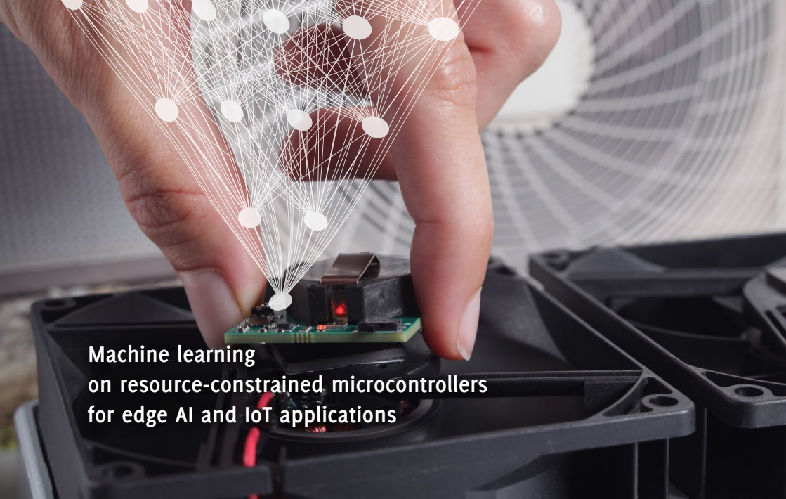
Figure 1: At IMMS, algorithms for embedded systems were designed, optimised and implemented in a demonstrator for AI-based fan monitoring using the machine learning approach TinyML: Motor bearings or fan blades can be directly monitored with the compact retrofittable solution. Defective parts are indicated directly via a red LED. Photograph: IMMS.
