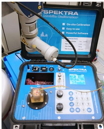
Figure 6: Measurement equipment for characterising the energy harvester using shaker and vibrometer. Photograph: IMMS.
