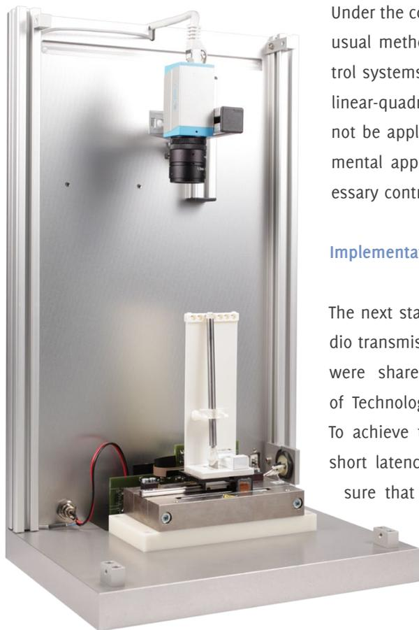
Figure 3: Equipment created at IMMS to demonstrate the inverted pendulum, including casing and integration of all control parts. Photograph: IMMS.
