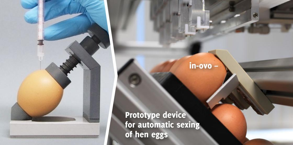
**Figure 1:** Commissioned by the VPCI of Leipzig University, IMMS has created a prototype device (right) for automatic sexing of eggs. The starting point was the specifications from VPCI experience with manual devices (left) configured for individual testing. Photograph (left): Professor Almuth Einspanier and Dr. Anne Weißmann. Photograph (right): IMMS.
