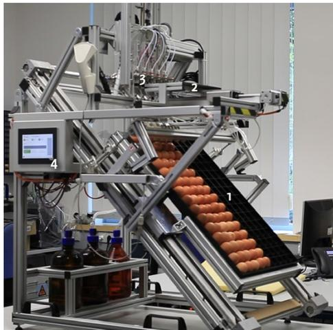
Figure 3: In-ovo tester made by IMMS, Prototype 1.0: (1) holder for one tray (15 rows, 5 filled columns for 75 eggs), (2) holder and actuator for titer plates, (3) puncturing module, (4) display and operating unit. Photograph: IMMS.
