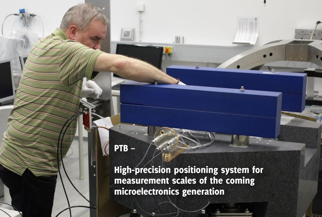
Work at IMMS for the Physikalisch-Technische Bundesanstalt (PTB) on a nanometre-precision planar drive system for a large travel range and use in vacuum. Photograph: IMMS.
