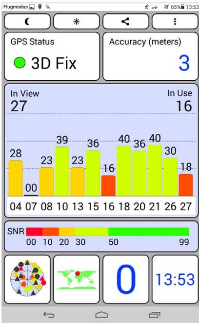
Figure 5. The quality of signal transfer from the frontend to a commercial available Android GPS device with the appropriate app was proved in a shielded measuring lab at IMMS. Signals from 16 satellites were received and decoded. The location was determined at an accuracy of 3m. Image: IMMS.
