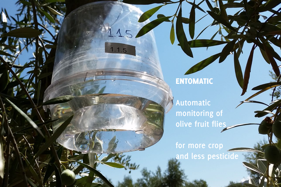
Figure 1: McPhail trap in original form as basis of an automatic monitoring of olive fruit flies. Photograph: Nutesca S.L., Spain.
