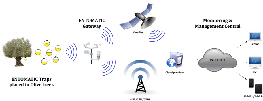
Figure 3: Schematic diagram of the ENTOMATIC system. Diagram: ENTOMATIC Consortium.
