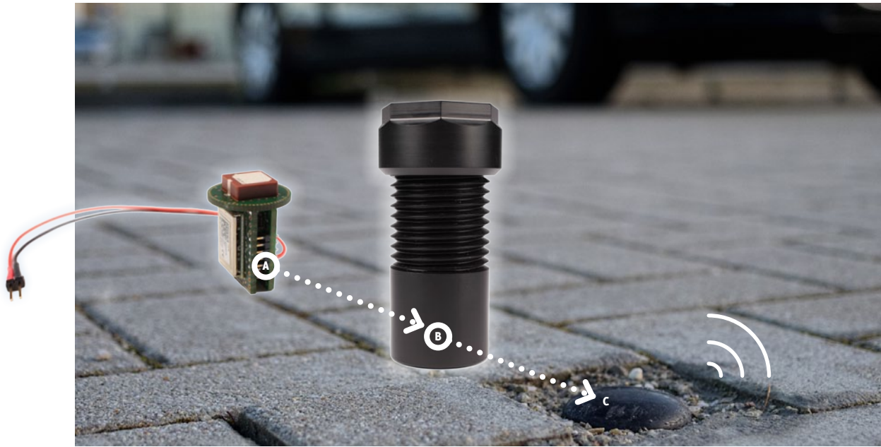
Fig. 1: The electronic detector module (A) developed by IMMS for insertion into the sensor pod (B) installed in the "tactile road" (C). Photographs: IMMS.
