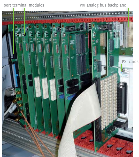
Fig. 3: Test setup showing IMMS MTS-1 and the connecting wires to the testing card. Photograph: IMMS, Industrial Electronics and Measurement Technology.
