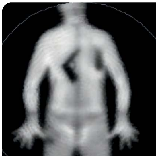
Figure 1: Image left: objects tested (mock pistol, 65g tartaric acid and ceramic knife) Image right: output from the first generation THz Scanner Photographs: IPHT Jena.
