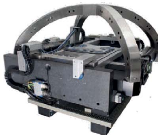
Figure 3: Air-guided 3D Direct Drive, Driving Area 400 x 400 mm 2 , Source: IMMS 2009
