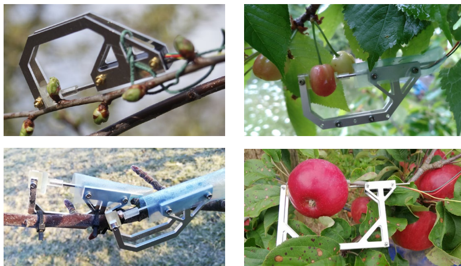
Figure 4: This dendrometer, developed in various versions as part of the EXPRESS project at IMMS, was used to monitor bud growth (top left) and the stone-hardening phase in cherries (top right), to monitor bud growth in the context of late frosts (bottom left), and for studies into the influence of soil cultivation on fruit quality (bottom right). Photograph: IMMS.
