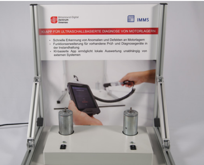
Demonstrator developed at IMMS at the SME Digital Centre Imenau for ultrasound-based diagnosis of motor bearings with AI-based data evaluation in an app.
