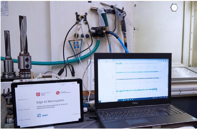
Flexible data acquisition solution for AI-based industrial applications. With the electronics platform, multi-channel measurement and training data can be recorded in industrial manufacturing environments for various questions and evaluated with the help of AI.
