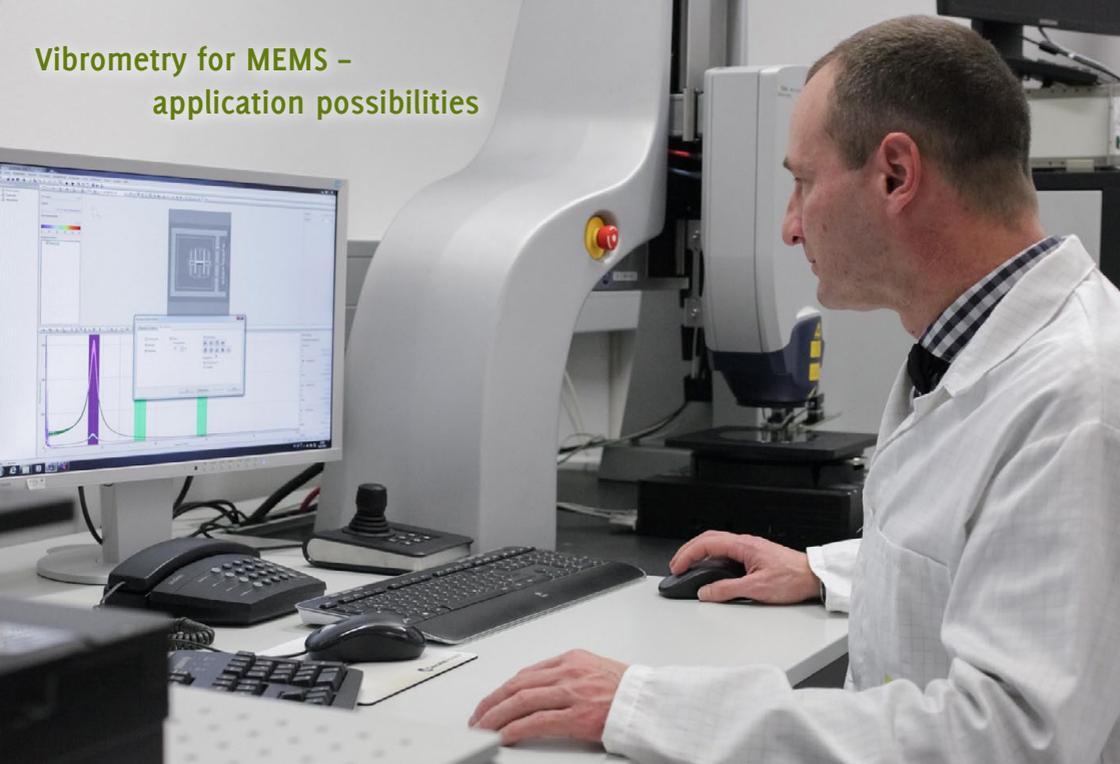
Measuring workstation for the acquisition of 3D vibrations on MEMS. Photograph: IMMS.
