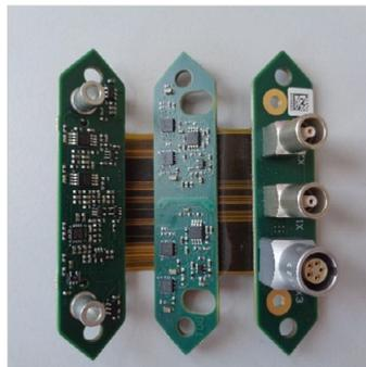
Figure 1: 3D representation of the three-channel extension boards for the SONAPHONE® and realised hardware. Diagram: IMMS, photograph: SONOTECH.
