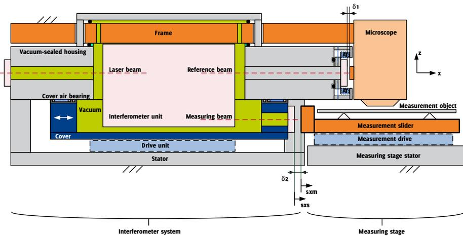
Simplified sectional view of the interferometer system with an exemplary embodiment of a sealing arrangement and a coupled measuring stage. Diagram: IMMS.
