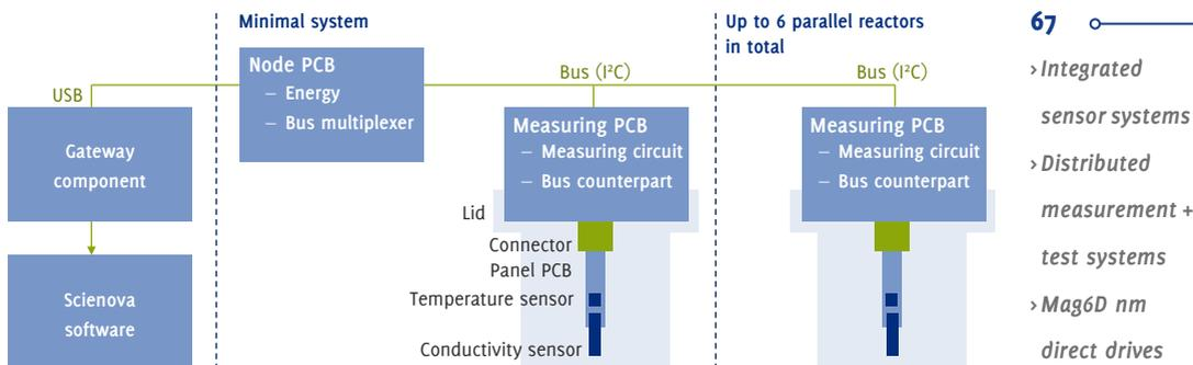
**Figure 2:** Concept of a sensor system for online monitoring of reactions in membrane reactors. Diagram: IMMS.
