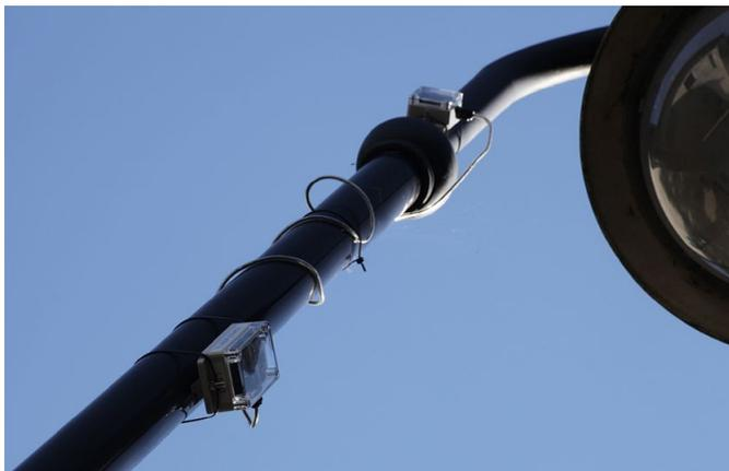
Sensor node prototype installed in Ilmenau for automatic lamp monitoring with radio communications as the first SmartCity test setup by IMMS in the thurAI project.
