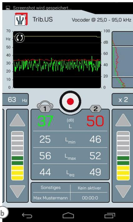
Figure 2: Trib.US app interface with (a) display of the frequency components in the ultrasonic range and (b) the level curves of two synchronous channels/sensors for test objects, e.g. roller bearings, as well as the third reference channel with the rotation speed. Source: SONOTEC.
