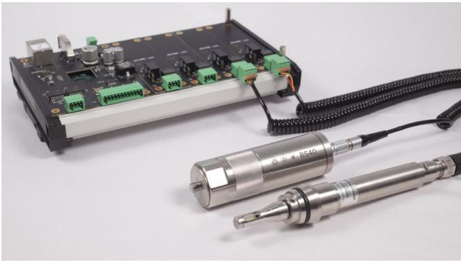
The sUSE hardware platform for compressed air monitoring with ultrasonic sensor from SONOTEC (left) and volume flow sensor from Postberg (right).
