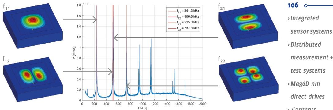
Figure 2: A frequency response function (FRF) with split frequency peaks. Diagram: IMMS.
