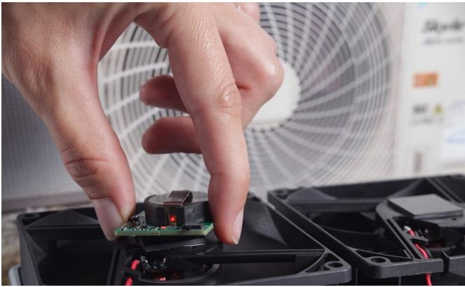
The retrofitable AI-based sensor for fan monitoring is a small sensor system that detects, classifies and visualises defects on fan blades or bearings. The sensor signal evaluation is made with an AI-based data processing implemented on a microcontroller.
