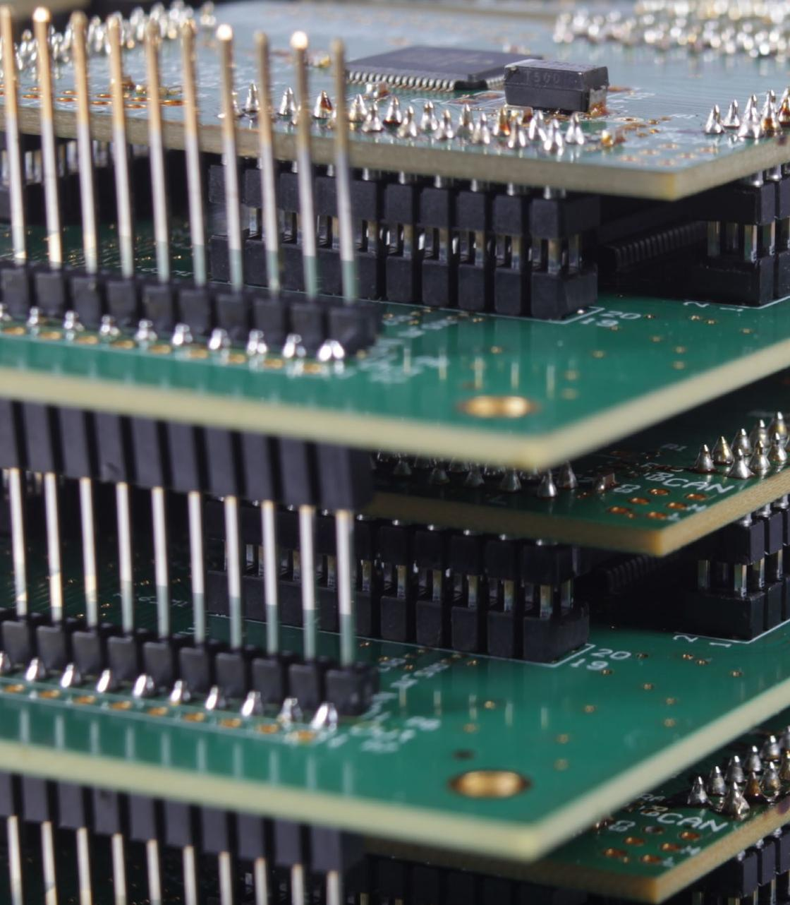
Modular measurement environment for mixed-signal real-time parameter acquisition during life tests. It enables time- or cycle-based tests at up to 175 °C on up to 128 components simultaneously. Photograph: IMMS.
