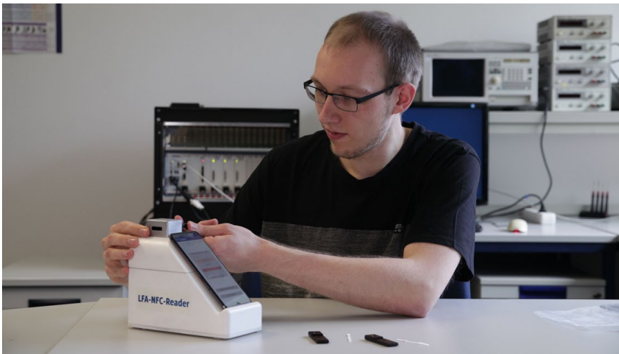
Markus Ismer with his demonstrator for the energy-autonomous read-out of LFA test strips via NFC. Photograph: IMMS.
