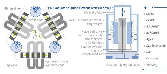
**Figure 3:** schematic representation of a planar drive system with 3 pairs of coils.For the 6-DoF drive, instead of the 3 air-bearings, 3 vertical drives (right) were installed. Diagram: IMMS.
