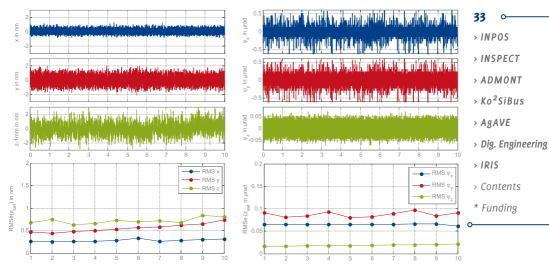
**Figure 6:** Time signals from the six coordinates in controlled operation (left); RMS control deviation in dependence on levitation height z<sub>set</sub> (right). Graphs: IMMS.
