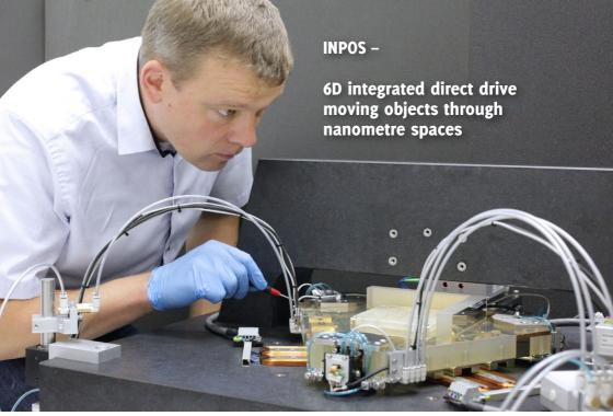
Work on a 6D direct drive capable of positioning objects anywhere in an area of  $\varnothing$  100 mm while raising or lowering them through 10 mm under active control on the nanometre scale. Photo: IMMS.
