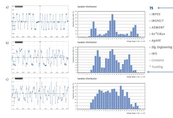
**Figure 4**: Comparison of Ethernet signal and associated distribution when affected by parasitics, shown under the influence of (a) normal conditions (clarity=531, asymmetry=53), (b) parasitic capacitance of 47pf (clarity=450, asymmetry=129) and (c) parasitic capacitance of 100pf (clarity=362, asymmetry=151). Source: IMMS.
