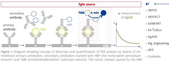
enzyme) and TMB (tetramethylbenzidine) substrate solution. The colour change caused by the HRP-TMB reaction alters the luminous intensity, which is what is measured by the chip. Diagram: IMMS/ Senova.
