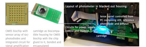
Figure 2: The optoelectronic CMOS biochip (left) which is exchangeable because of the cartridge solution (centre) can be used in the photometer for the analysis (right). Photographs: IMMS.
