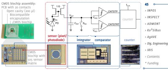
Figure 6: Photograph of the chip and circuit diagram, D4021A CMOS biochip. Photographs and diagram: IMMS.
