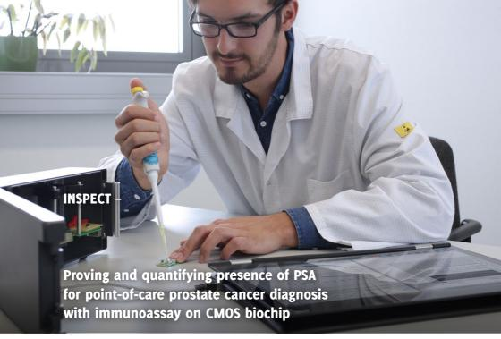
Senova and IMMS are the first to succeed in precisely quantifying PSA (prostate-specific antigen) directly with an opto-electronic CMOS biochip by measurement of light absorption. The method fully complies with "Rili-BÄK", the guidelines published by the German Medical Association (Bundesärztekammer) for quality assurance in medical laboratory tests. Photograph: IMMS.
