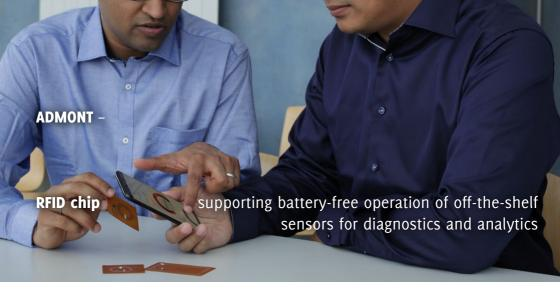
IMMS has developed an RFID sensor transponder IC as a bridge between NFC and I<sup>2</sup>C, with which commercial sensors for diagnostic and analytical applications can be connected and operated without batteries. Photograph: IMMS.
