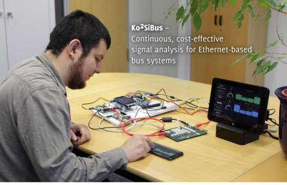
IMMS has developed novel cost-effective methods of monitoring data lines across running industrial plant. A demonstrator maps the entire system with the complete analysis chain: Ethernet signals can thus be manipulated in a targeted manner to simulate cable faults artificially or to show the influence of such faults. Photograph: IMMS.
