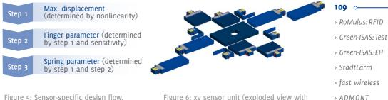
Figure 5: Sensor-specific design flow. Diagram: IMMS.
