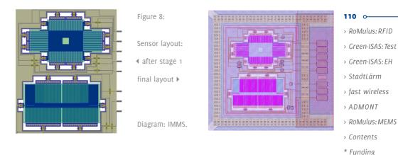
contacts and connects them to the pads is carried out manually except where wires cross. The "crossing" layout element is always inserted automatically. In the second step, the X-FAB process design kit is used to add further layout elements specific to the fabrication technology.
