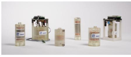
Figure 5: Selection of demonstrators (versions top left and top right have frontend circuits and wireless sensor circuits). Photograph: IMMS.
