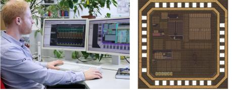
Figure 3: Working on the layout (I.) of the D8016B research ASIC (r.) which contains ULP circuits
