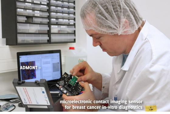
IMMS has developed an opto-electronic testing system to enable precise diagnosis of breast cancer. The prototype is currently being employed by Oncompass Medicine Hungary Ltd. for investigations using cell samples. Photograph: IMMS.
