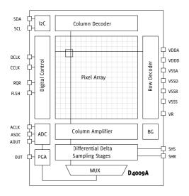
Figure 3: schematic circuit diagram of the imaging sensor. Diagram: IMMS.
