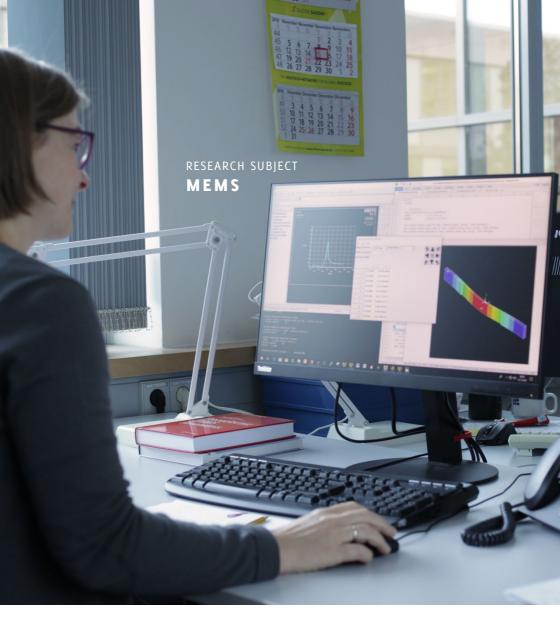
IMMS is a part of the MagSens research group working on MEMS sensors which will in future be capable of detecting weakest magnetic fields, such as those found in biomedical technology. The image is of one of the simulations, using ANSYS, of the transfer characteristics of a magneto-strictive piezoelectric MEMS beam structure. Photograph: IMMS.
