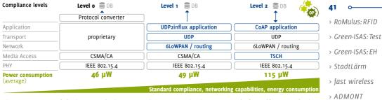
Figure 5: Stages of design complexity supporting communications protocols for self-powered wireless sensors in conformity with Industry 4.0. Diagram: IMMS.
