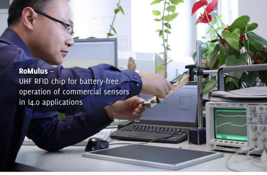
Carrying out measurements on the energy-efficient UHF RFID sensor transponder chip. This chip is for operating without use of a battery a variety of commercially available digital I<sup>2</sup>C sensors requiring varied power levels. Photograph: IMMS.
