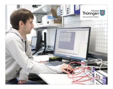
In the TSN laboratory\* funded by the "Land" of Thüringen, IMMS investigates technological limits in the development of dataintensive industrial real-time applications. For example, the behavior of the TSN Time Aware Shaper according to IEEE-802.1Qbv is analyzed with TSN development systems from the company NXP (front right) and methods for simplified parameterization of TSN networks are implemented (see the Monitor). Photo: IMMS.
