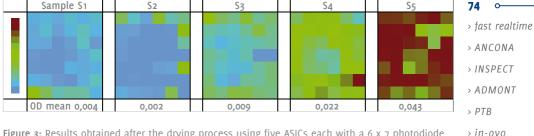
**Figure 3:** Results obtained after the drying process using five ASICs each with a 6 x 7 photodiode matrix for solutions S1 to S5 containing nanoparticles of gold: blue marks the lowest, green the mean and red the maximum value for optical density (0D, in Bel). The "0D mean" values shown are the values for each ASIC for optical density. Diagram: IMMS.
