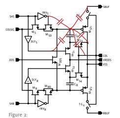
Existing tools reveal the problem but are unable to identify the parasitic elements leading to the error.
