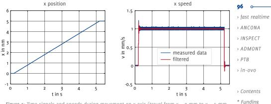
**Figure 5:** Time signals and speeds during movement on x axis (travel from x = 0 mm to x = 5 mm,  $v_{soll}=1 \text{ mm/s}$ , RMS deviation in speed: 4.2  $\mu$ m/s<sup>\*</sup>) 4,2  $\mu$ m/s<sup>\*</sup>) \*Filter used for determining speed: bandpass filter with pass up to 200 Hz, stop after 300 Hz. Diagrams: IMMS.
