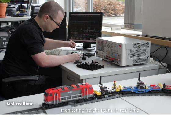
Energy demand measurements on prototypes for a low-latency train monitoring system with local radio sensor network. Photograph: IMMS.
