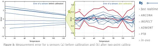
tion at 20°C and 100°C; the red line relates to the average tolerance of  $3\sigma$ . Diagrams: IMMS.
