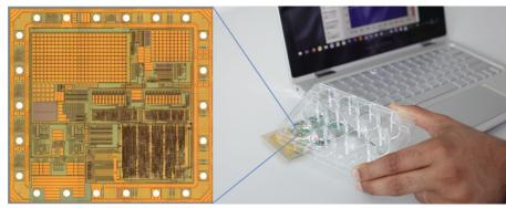
Figure 3: Passive HF RFID tag with integrated temperature sensor (left: photograph of chip; right: RFID tag with chip on the RFID antenna coil, in use for measurements in a liquid). Photographs: IMMS.
