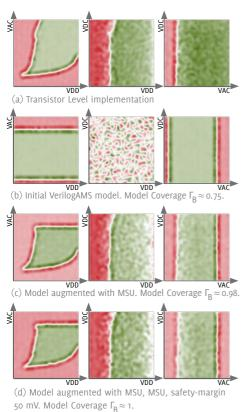
Figure 11: comparison of the circuit and model acceptance regions with and without MSU. Diagram: IMMS.
