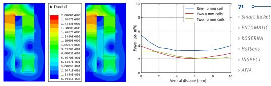
Figure 4: FE analysis of one version of the electromagnetic actuator with single-phase (l.) and two-phase (centre) coils; also shown is the heat loss calculated for a set distance of 10 mm carrying a load of 50 g (r.). Diagrams: IMMS.
