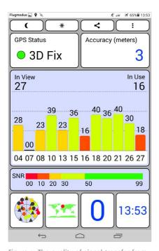
Figure 5. The quality of signal transfer from the frontend to a commercial available Android GPS device with the appropriate app was proved in a shielded measuring lab at IMMS. Signals from 16 satellites were received and decoded. The location was determined at an accuracy of 3m. Image: IMMS.
