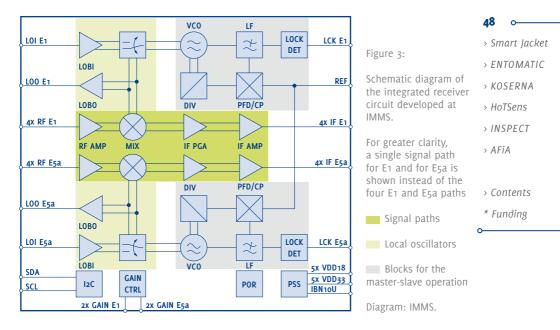
oscillator on the eight paths in each frequency band. For each of these bands there is a frequency synthesiser on the chip. The two chips are configured so flexibly from a digital interface (I<sup>2</sup>C) that at any one time only one chip acts as frequency synthesiser on behalf of both, creating the local oscillators and distributing them to the second chip. It is this master-slave arrangement that makes coherent frequency conversion feasible for all the channels.
