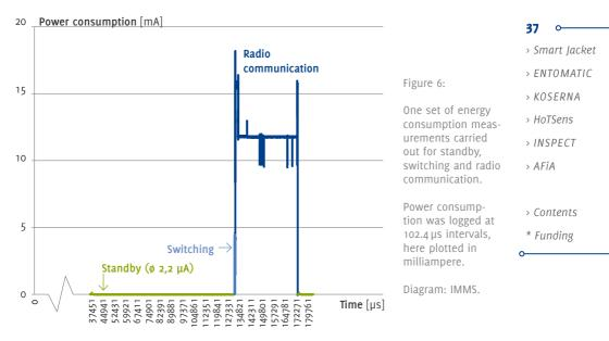
nied the development process and were carried out for the main operating phases: assignment of switches to devices, standby and switching followed by radio communication, see Fig. 6.
