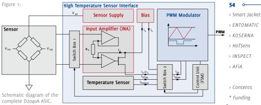
Areas exposed to espeacially strong temperature effects are marked in red. Diagram: IMMS.
