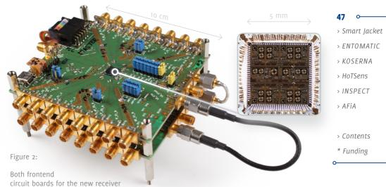
together with 2 SMA connectors per channel will fit onto an area 10 cm square situated beneath the group antenna. At the centre of each board there is an ASIC (5 x 5 mm<sup>2</sup>, see detailed graphic) sealed directly onto the board (Chip-on-board technology). Photograph: IMMS.
