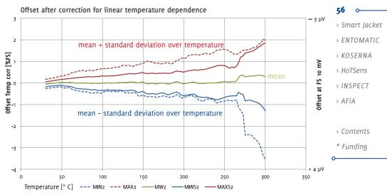
Figure 4: Measurements at accuracy of  $\pm 1.5$  % FS (FS being full scale). Diagram: IMMS.
