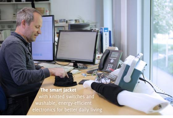
This desktop experimental setup with a breadboard was used to put the principles of the smart jacket to the test, particularly the control of the outside devices from the switch patches, and use of smartphone to configure. Photograph: IMMS.
