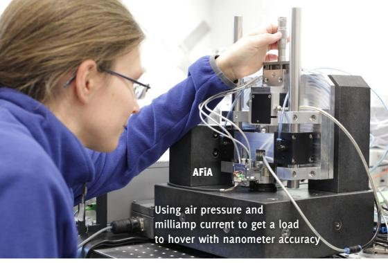
IMMS has developed a vertical drive to raise and lower objects through 10 mm under active control with nanometre precision. Photograph: IMMS.
