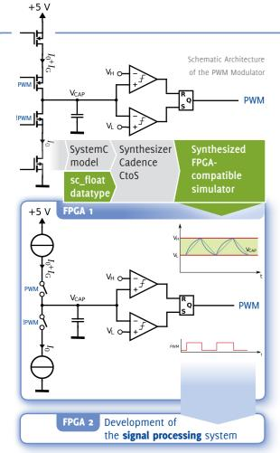
Fig. 5: Simulation of a mixed-signal system using the FPGA method. Diagram: IMMS.
