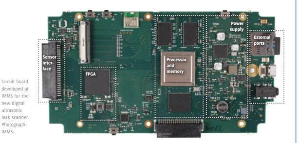
age of test data, levels and spectrograms, generation of test reports and camera documentation of leaks. To transmit data efficiently and to enable the data to be integrated into existing systems, the device uses interfaces like Bluetooth, USB and SD/MMC.
