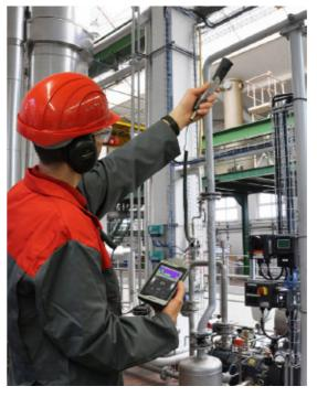
The newly developed ultrasonic detector in use for preventive maintenance purposes. The device was launched at the 2016 Hannover Messe. Photo copyright: fotolia: industrieblick/SONOTEC.
