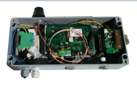
Figure 3: Environmental sensor exposed to show power supply, gateway electronics and sensor system (on boards from left to right). Photograph: IMMS.
