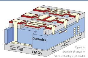
of a MEMS-based multi-frequency oscillator on a SiCer substrate with hybrid integration. Source: TU Ilmenau / IMN MacroNano.
