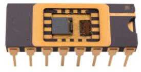
Fig. 5: One of the modules with encapsulated acceleration sensor (l.) and signal evaluation ASIC (r.) set up for the investigations on the shaker. Photograph: IMMS.
