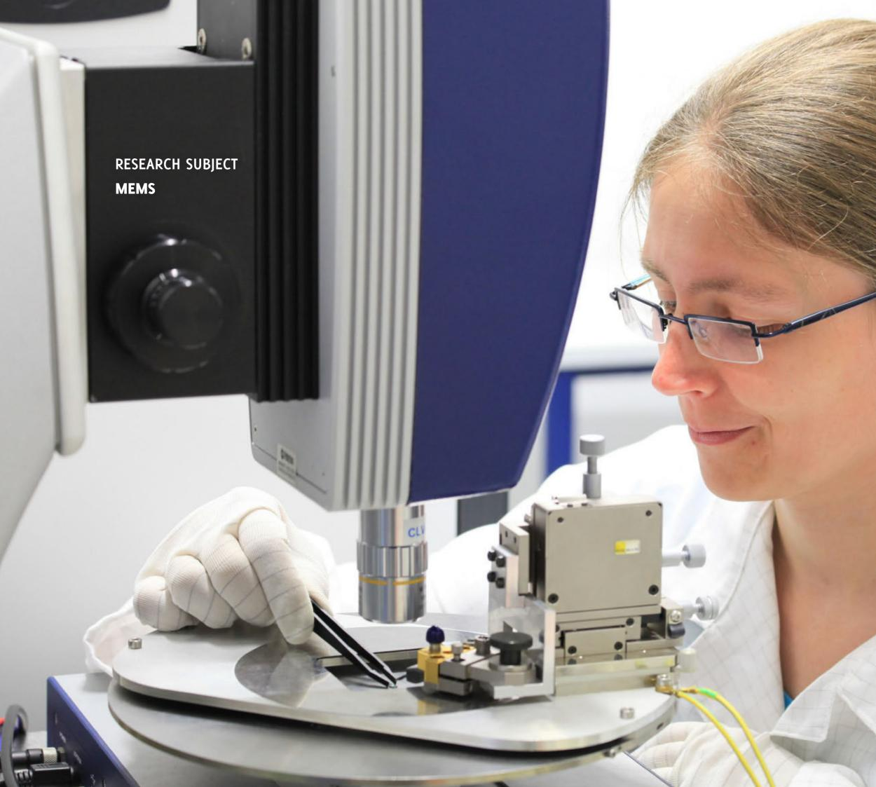
Preparing vibrometry experiments on encapsulated MEMS structures. IMMS has been working in the IRIS project since 2015 on new measurement methods intended to enable quality testing of encapsulated MEMS during manufacture. Photograph: IMMS.
