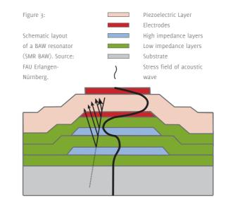
filter, besides these frequency changes due to the environmental conditions, there is also warming of the filter due to the signal current, which changes the behaviour of the filter. A further complication is the variability due to manufacturing processes. This may also reduce the effective band gap. These potential problems render indispensable the precise modelling of the temperature-related behaviour of the filters.
