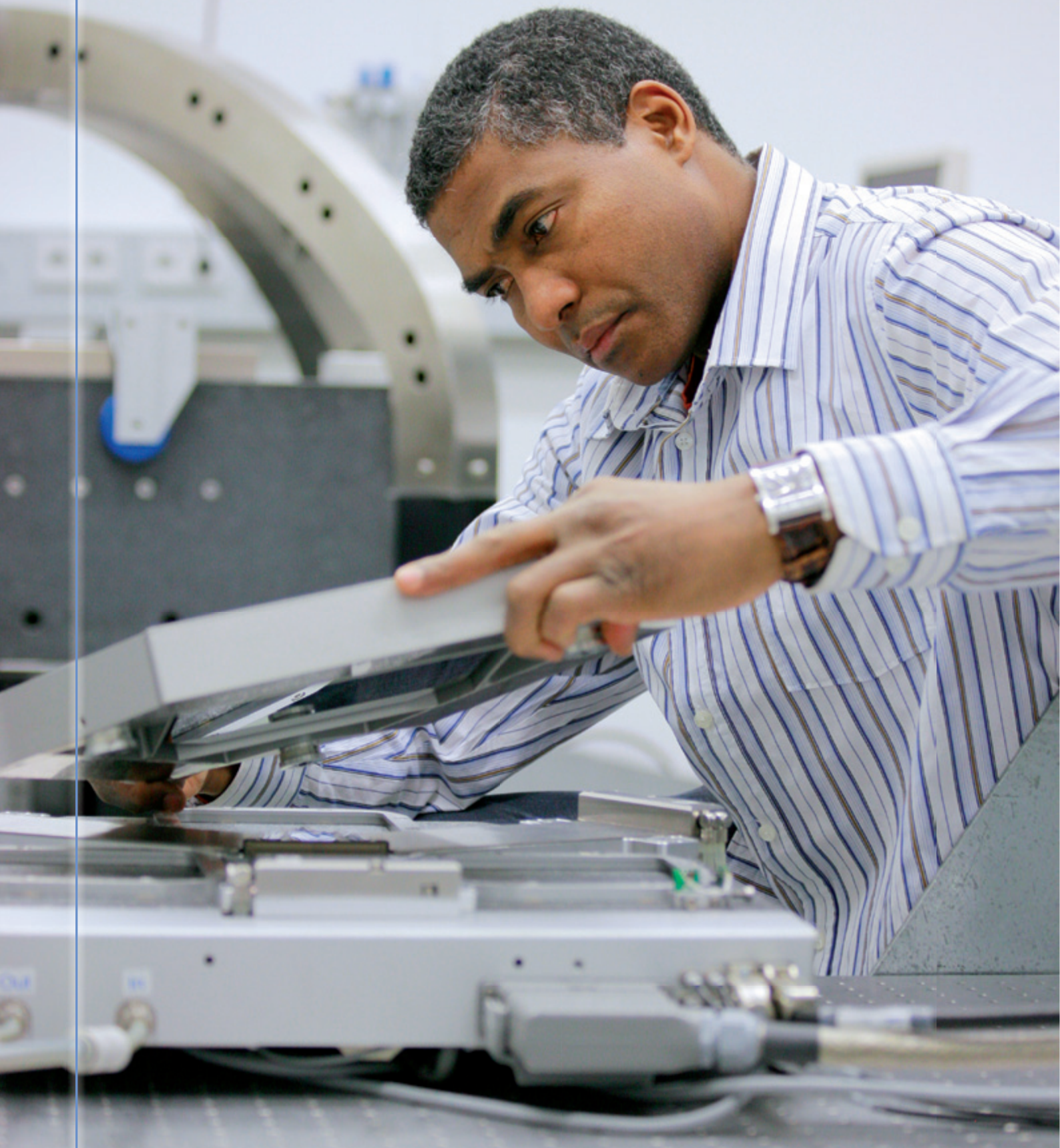
Maglev direct drive with passive stage and no wiring. Photograph: IMMS.
