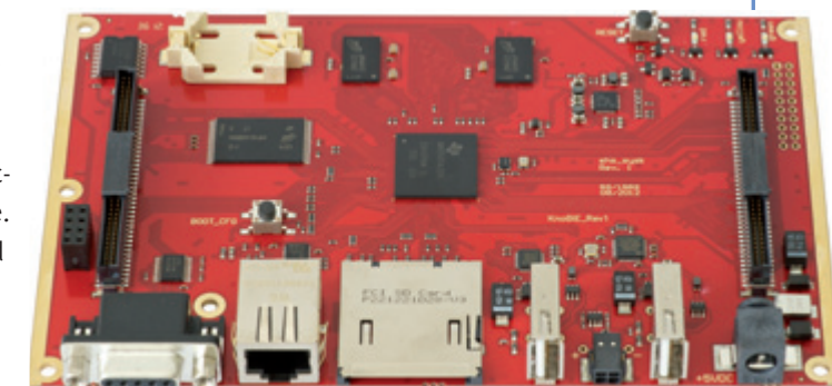
Figure 2: Base board of the SHS system node. Photograph: IMMS.
