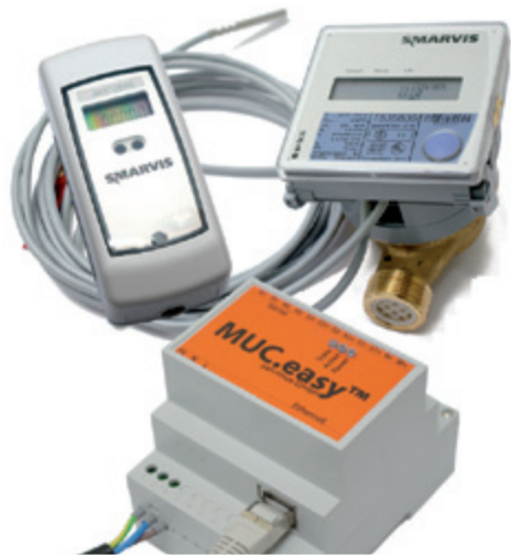
Figure 3: Wireless water and heating meters and a smart meter gateway. Photograph: IMMS, System Design.
