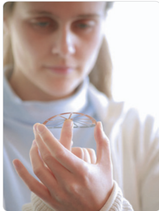
Figure 3: The vertical motion of the smart pixel camera is stabilised by three membrane springs. Source: IMMS
