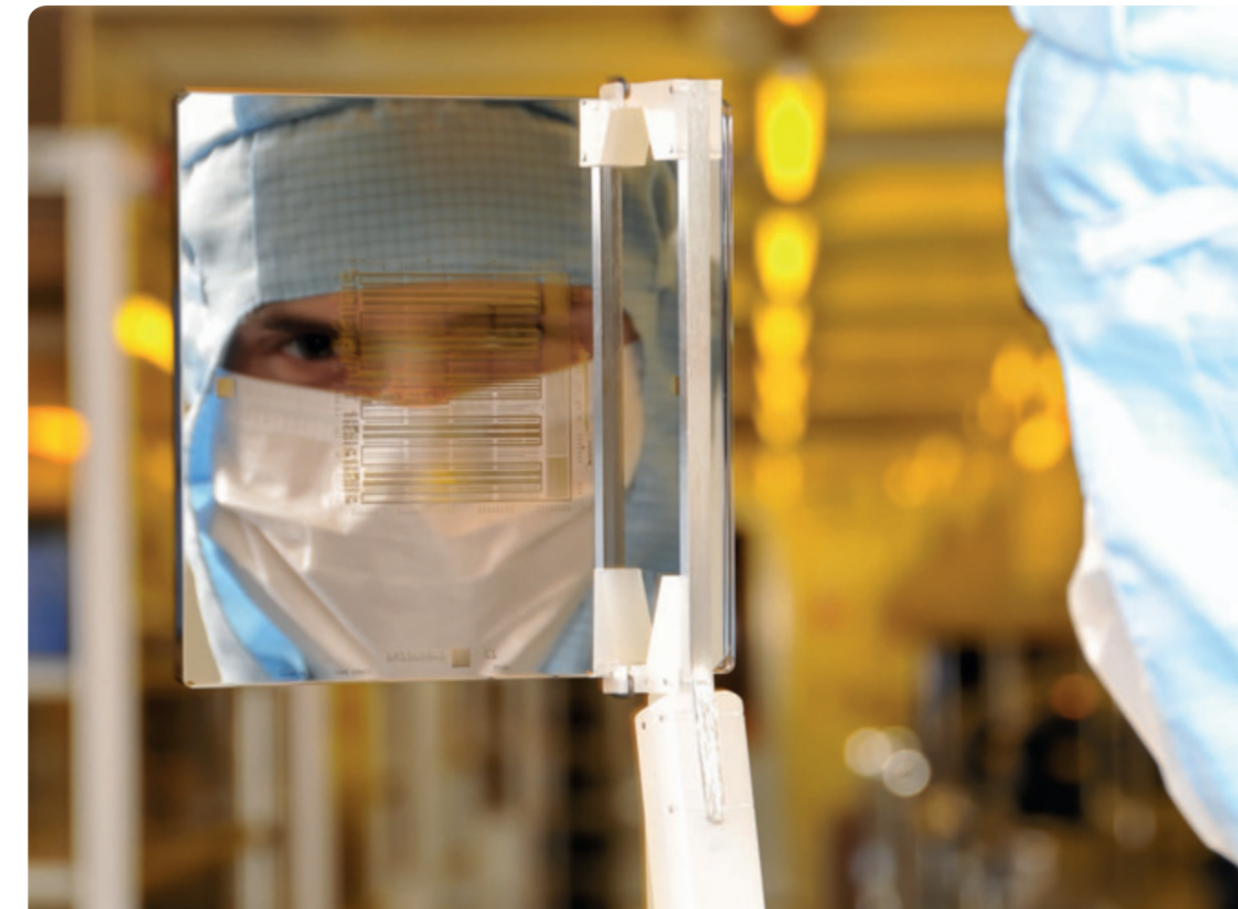
Figure 1: Reticles like this are used in semiconductor production to transfer circuit structures to the photo layer of a wafer. These structures are based on the circuit design. Source: X-FAB AG/Michael Voigt.
