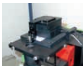
fig. 1: XY table at the wafer prober with optical fibre coupling
