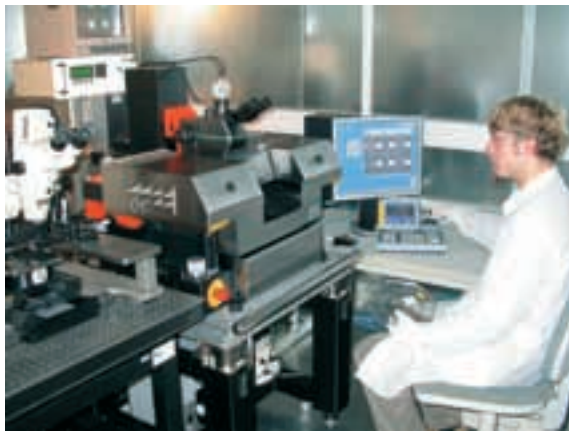
fig. 1: Semiautomatic wafer prober PA200 in shielded cabin
