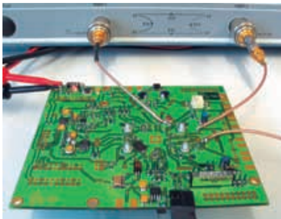
fig. 1: Evaluation board of an RF ASIC connected to a VNA
