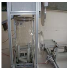
Fig. 2: experimental setup of wafer illumination module (source: TU Ilmenau)
