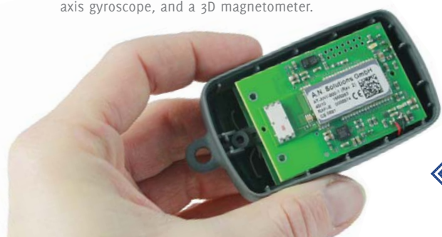
Example of a MEMS energy harvesting device for self-powered operation of microsensor systems.
