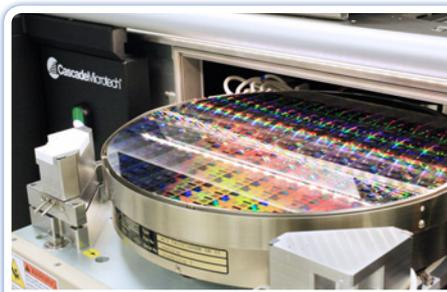
Measurement of a sensor ASIC at device level
