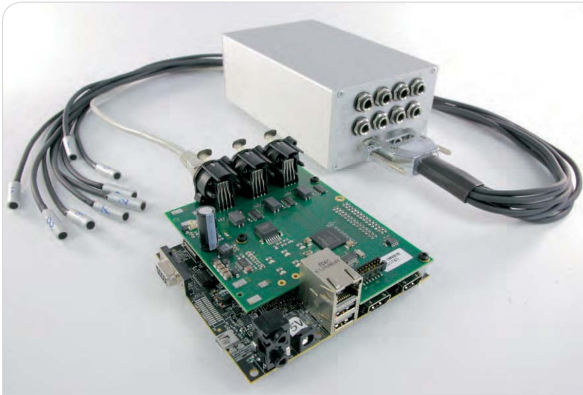
The "S4ECoB" system, consisting of a microphone array and an embedded energy-efficient hardware and software platform. The system is capable of determining the number of people in parts of a building based on acoustic data and control building systems accordingly. Photograph: IMMS.
