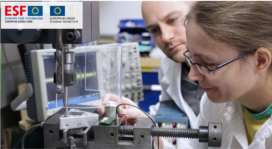
Initial experiments on energy harvesting in the Green-ISAS project to supply energy to sensors in industrial plant. Photograph: IMMS.
