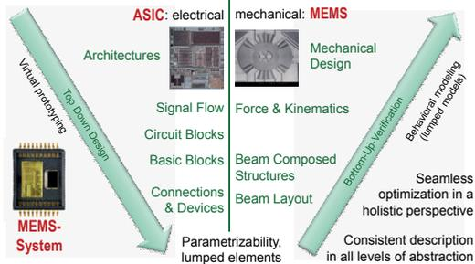
In the end this leads to a seamless, Lego-brick-style design-flow for heterogeneous systems, offering enormous simplicity. Electrical and mechanical systems can be simultaneously described, simulated and designed in one model, leading to a faster development of the final application.
